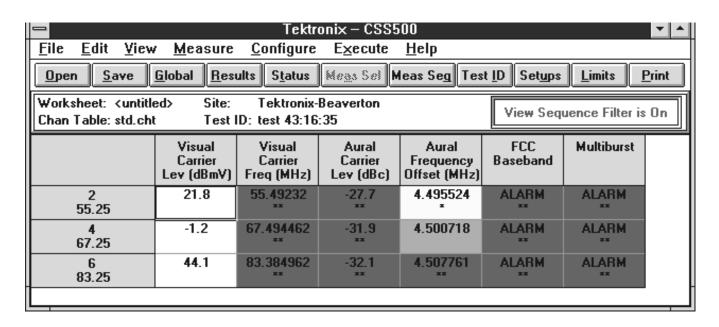
Figure 2–30: Measurement sequence results with view sequence filter on
