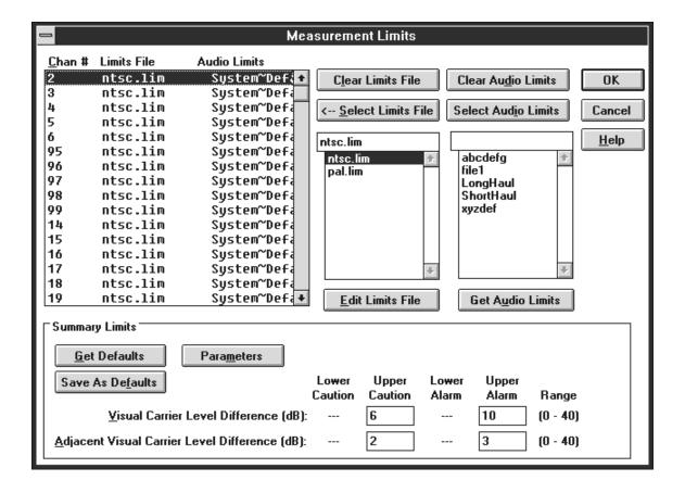
Figure 3-40: The Measurement Limits dialog box
