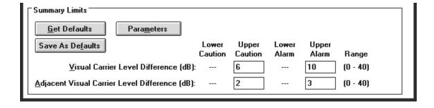
Figure 3–44: Summary Limits (part of the Measurement Limits dialog box)
