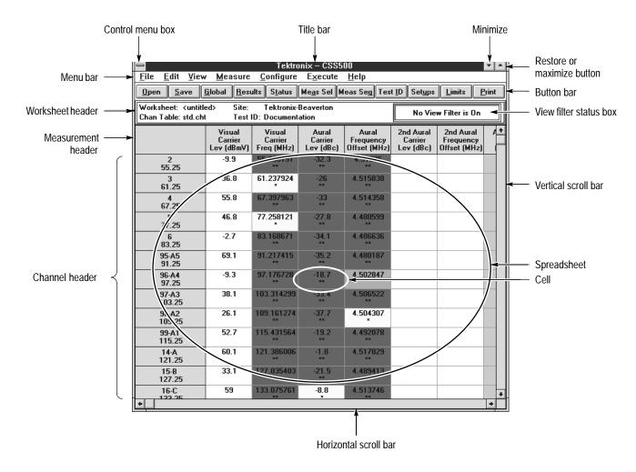
Figure 3-1: Parts of the CSS500 worksheet
