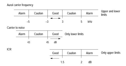
Figure 3–42: How the upper and lower limits work
