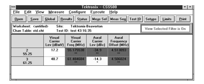
Figure 2-65: The Spreadsheet with the Measurement and Channels View Filter on
