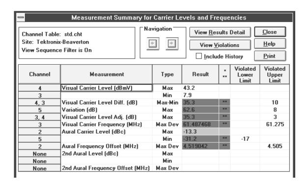
Figure 3–21: Example of a Measurement Summary
