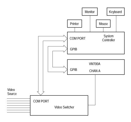
Figure F-4: Using a switcher
