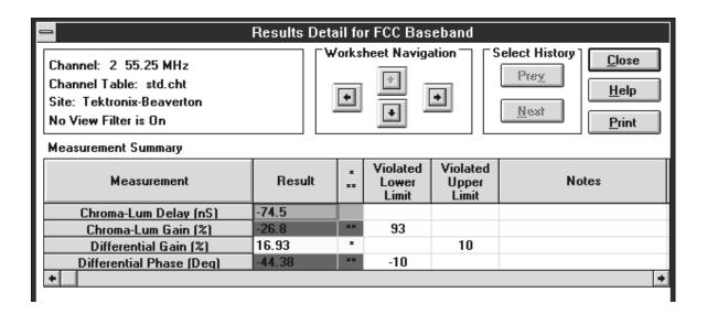
Figure 2–52: The Results Detail dialog box for the FCC Baseband measurement for the first channel
