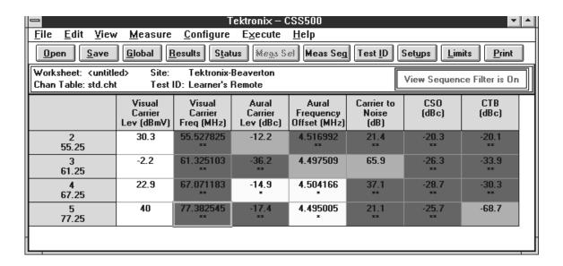
Figure 3-24: Worksheet with Measurements and Channel View Filter on
