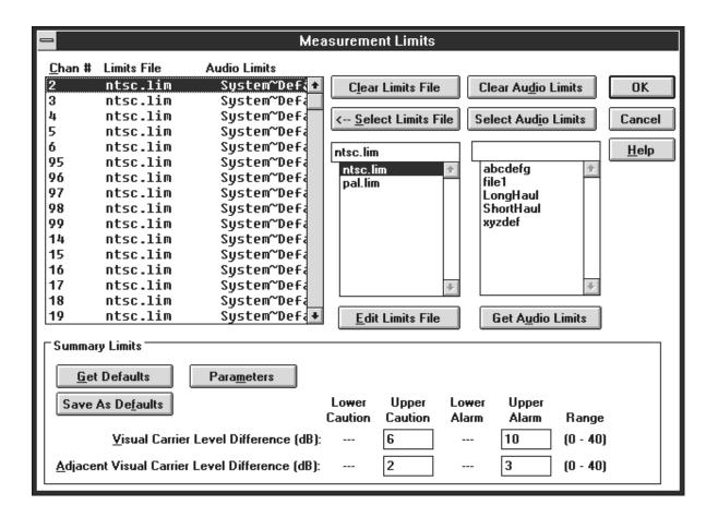
Figure 2–69: The Measurement Limits dialog box
