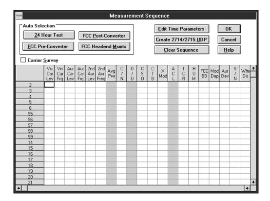
Figure 2–24: The Measurement Sequence dialog box (if operating country is United States)
